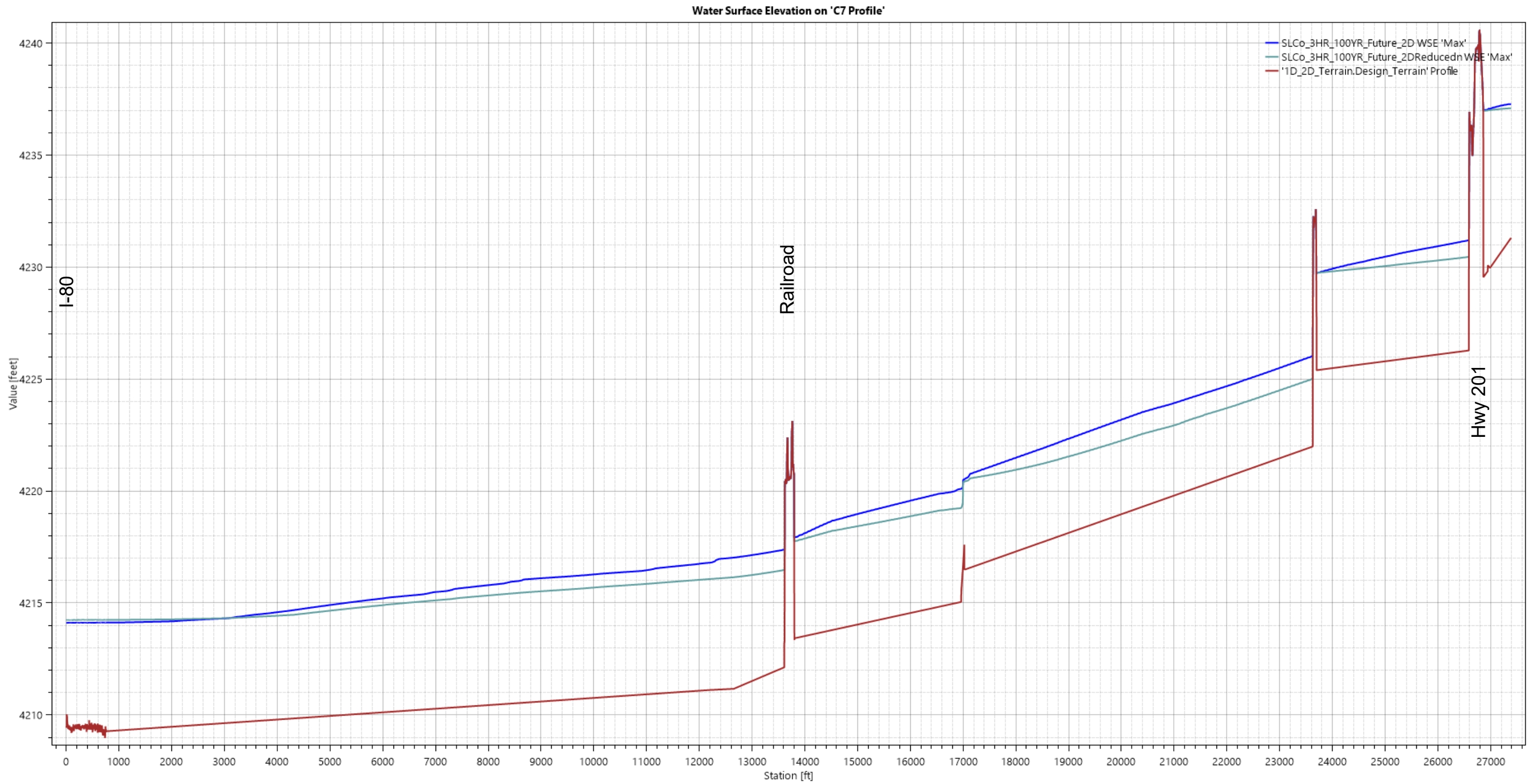
FIGURE III-12. C-7 Design Flow Profiles for Existing Channel Roughness (n= 0.06) and Maintained Channel Roughness (n= 0.035).
