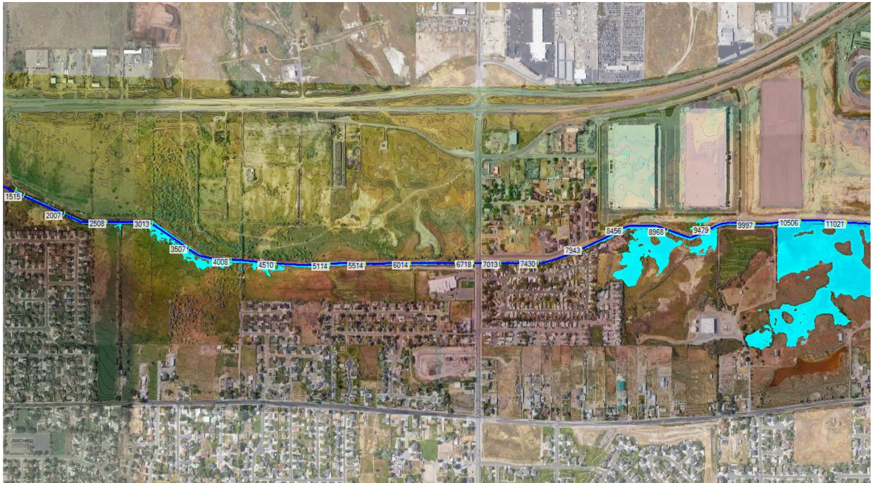
Figure VIII-6. Riter Canal Existing Conditions Plan View with Inundation Map for 10-Year Event (1 of 2).
